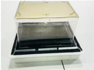
Place your plastic container upside down onto your metal plate. Fit the box so that the box walls fit the grooves in the metal plate. Now your chamber is ready to detect particles. It will only take a few minutes until everything has cooled down and a stable sensitive area has formed.
