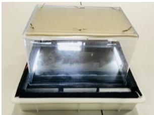
At first, you will only see a rain-like mist of alcohol. Place your torch lights in a way, that they illuminate the alcohol mist right above the metal plate – that is the sensitive area of the chamber.
