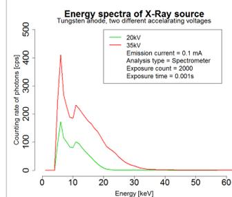
The energy spectrum of X-Ray machines with different acceleration voltages can be measured.
