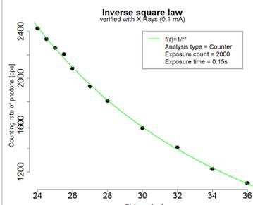
In the analysis type "counter" the MX-10 detector measures the number of particles. This can be used, for example, to verify the inverse square law.
