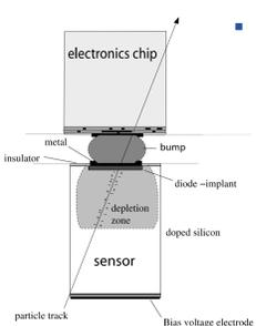
Cross section through one pixel with particle track [2]
