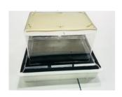
Place your plastic container upside down onto your metal plate. Fit the box so that the box walls fit the grooves in the metal plate. Now your chamber is ready to detect particles. It will only take a few minutes until everything has cooled down and a stable sensitive area has formed.
