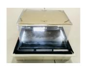
At first, you will only see a rain-like mist of alcohol. Place your torch lights in a way, that they illuminate the alcohol mist right above the metal plate – that is the sensitive area of the chamber.
